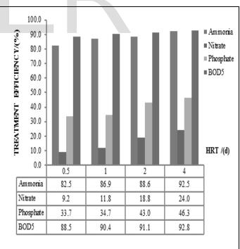
Fig. 3. Treatment efficiency of wastewater parameters in hybrid system of different HRTs
